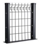
Bekafix® Secure posts are specifically designed and engineered to be used in combination with Betafence's panels. With Bekafix® Secure, the fence is safely tucked behind the lip of the post, withstanding attempts to pry the panel loose. The panels are secured to the post with specialised spider brackets, firmly bolted through the post using M8 stainless steel security bolts and shearoff nuts that protect against tampering.
