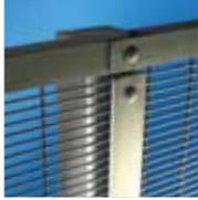
**Square post system:** For PVC coated panels only. The panels are fixed on the front side of the posts by means of fixators and security bolts. The welded square tubular posts (76 x 76 x 2 mm) have inserts for fixing the panels with the fixators and are covered with a plastic cap
