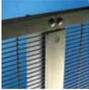
**Angle Iron Posts:** Posts are 70 x 70 x 6mm / 100 x 75 x 8mm (3000mm panel) are hot dipped galvanised in accordance with ISO-1461 and pre-drilled with holes for fixing panels, including (70 x 6mm) cover plate section with pre-drilled holes for fixing panels to posts. The panels are fixed to posts using stainless steel (M8 x 40mm) countersunk flushlock bolts and shear nuts.
